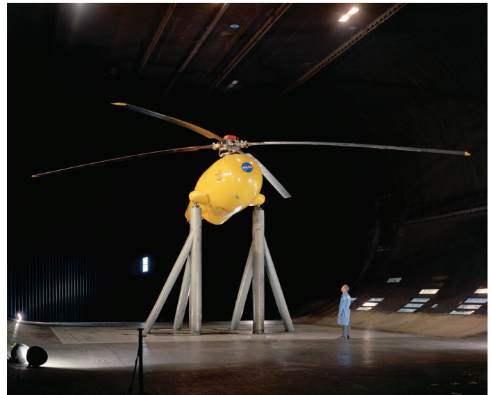
Figure A-14. CH-34 pressure-instrumented rotor in the 40- by 80-Foot Wind Tunnel (courtesy of NASA Ames Research Center).
