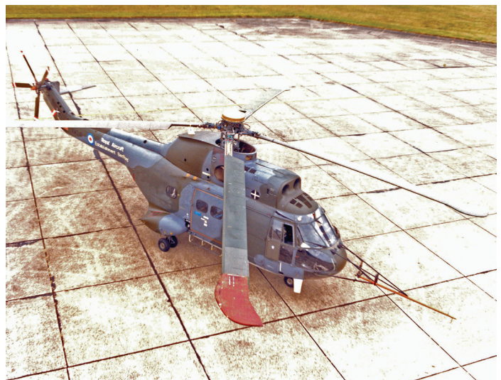
Figure 44. Research Puma with swept-tip blades at RAE Bedford.
