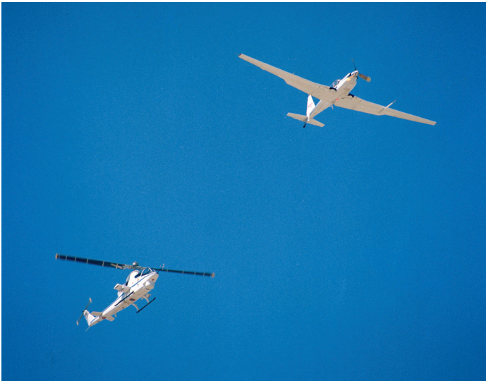
Figure A-41. AH-1G/TAAT airloads test aircraft trailing the YO-3A (courtesy of NASA Ames Research Center).
